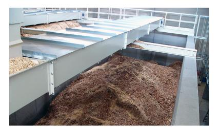
Bruks' drag-chain conveyors employ a heavy-duty chain and paddle transport arrangement that effectively traps and drags material between the paddles along the length of the conveyor to its end destination.
